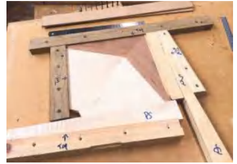
▲ Pic.14 To glue up these components, I built an adjustable jig to first glue an eighth of the face, which is two components, then a quarter, which is four components, and so on
